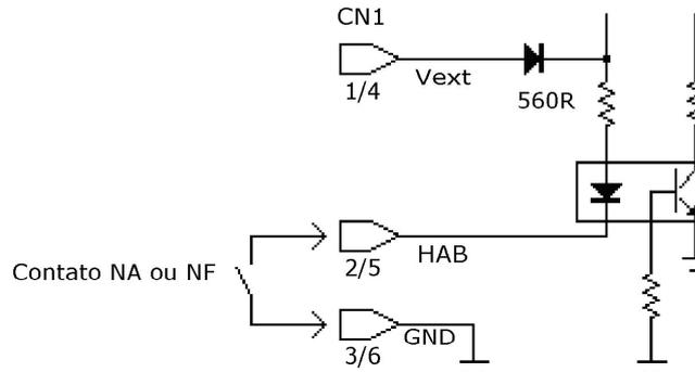
Enabling passage through tension pulse is shown in the image below. It is necessary to observe the polarity of the Vcc voltages and to use an external resistor for high voltages (110V and 220V).
