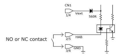
Enabling passage through tension pulse is shown in the image below. It is necessary to observe the polarity of the Vcc voltages and to use an external resistor for high voltages (110V and 220V).
