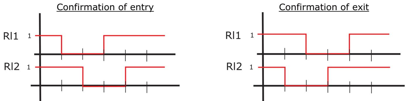
In this operation mode, any of the passage confirmation outputs – output RI1 or RI2 – can be used to activate an electromechanical counter in order to count the passage flow in both directions of the equipment.
