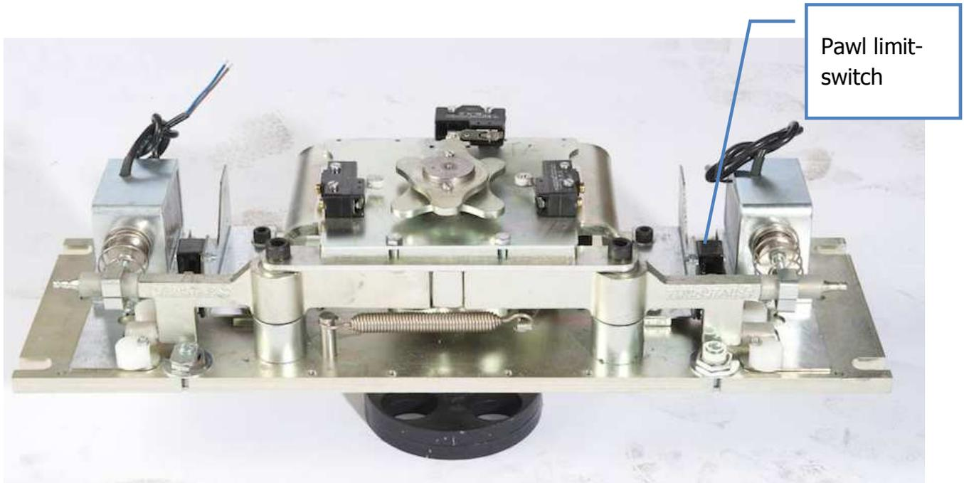
Figure 7.1: Mechanism image & pawl limit-switch
