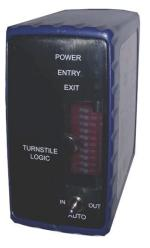
The TL300TUR is a turnstile logic unit which has been developed to control turnstiles using magnetic solenoid locks and limit switches. The TL300TUR accepts inputs from card readers or push buttons and performs all of the required timing and interlock logic.
