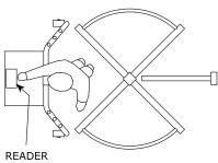
**STEP 3A:** READER CONFIRMATION - ACCESS ALLOWED TURNSTILE ROTATES A FURTHER 90° AND RELOCKS
