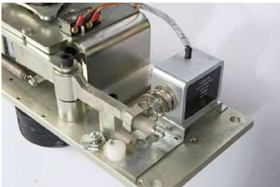
Figure 26: Solenoid in Fail-secure arrangement
