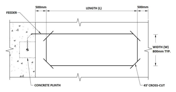
Figure 47: Loop Installation Plan View
