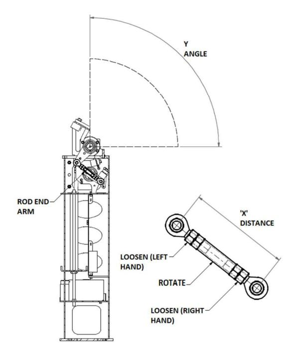
Figure 39: Rod End Arm Adjustment
