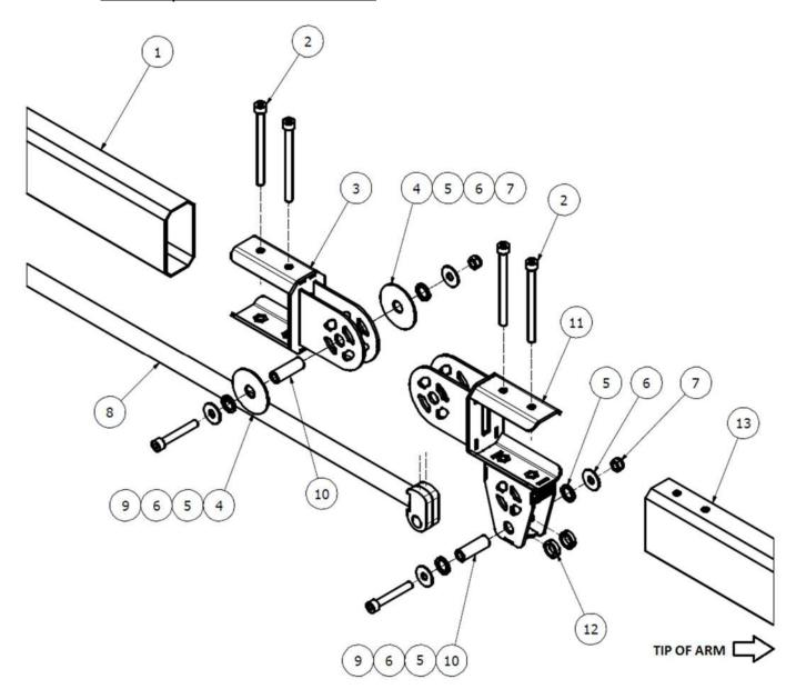
Figure 41: Articulated Arm Knuckle Assembly
