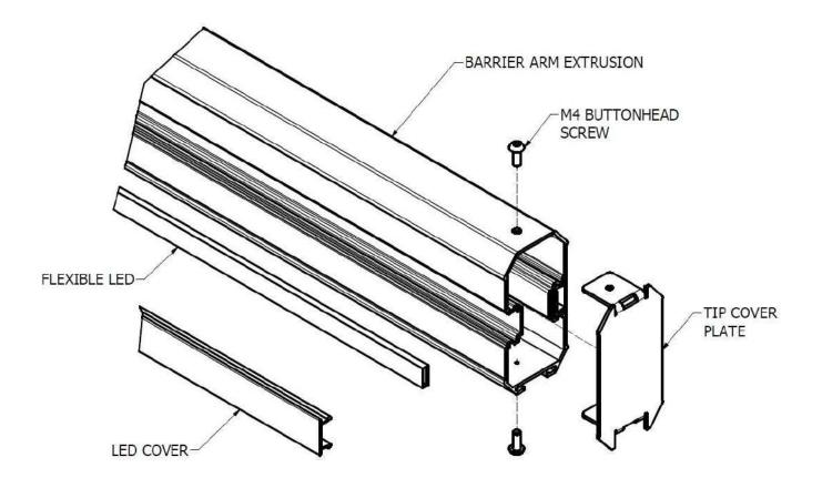
Figure 11: Barrier Arm LED and Tip Front Assembly
