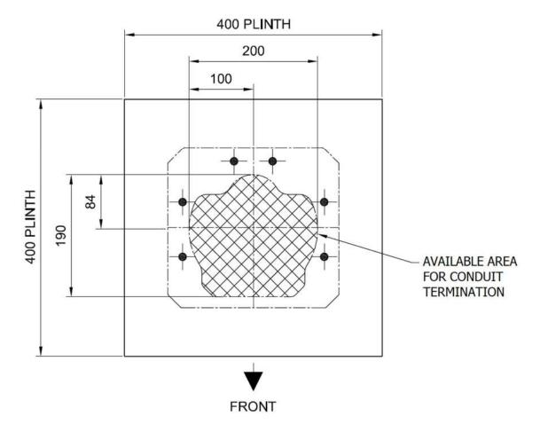
Figure 19: Plan View – Available Area for Conduit Termination
