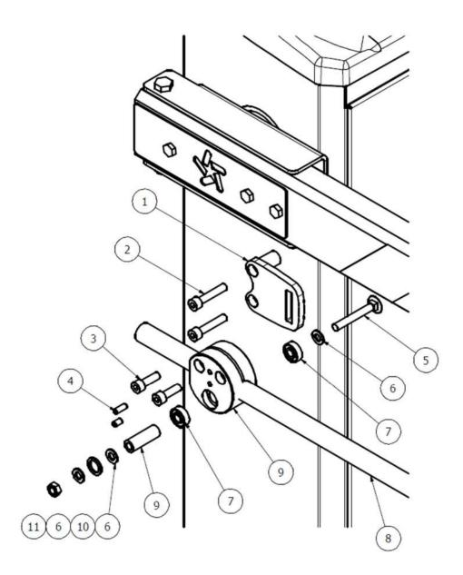
Figure 42: Articulated Arm Pivot Clamp Assembly
