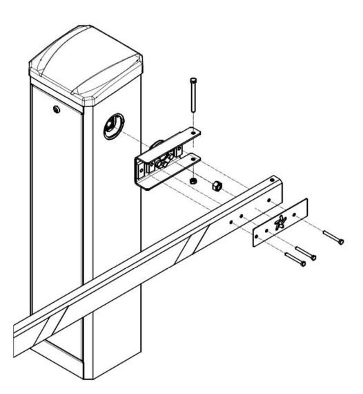
Figure 46: Replacing the Arm Clamp, Barrier Arm and Cover Plate (Left-Hand as shown)
