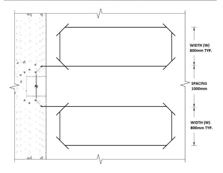
Figure 49: Loop installation example for Trucks
