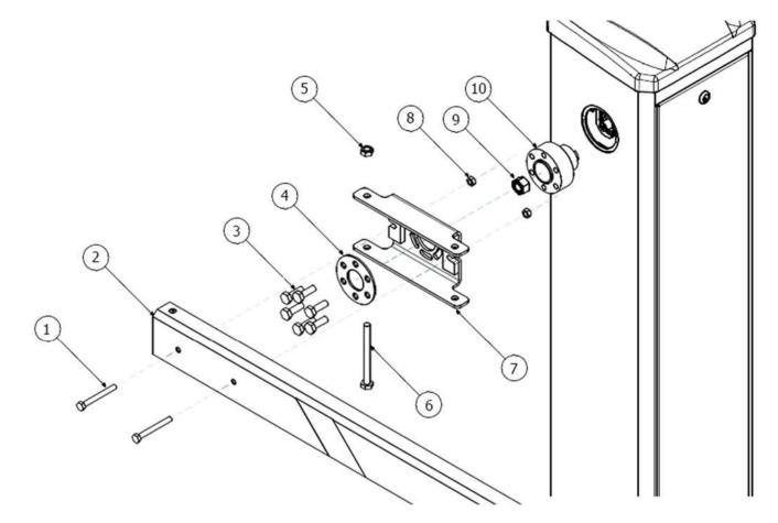
Figure 25: Removal of Barrier Arm Clamp Assembly
