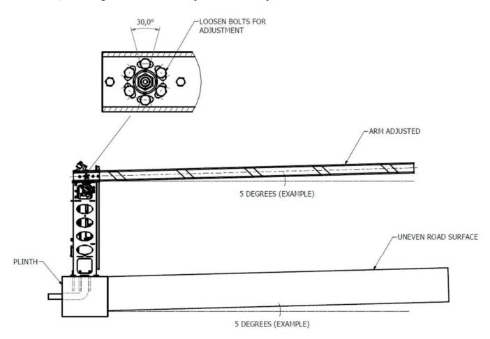
Figure 35: Barrier Arm Adjustment
