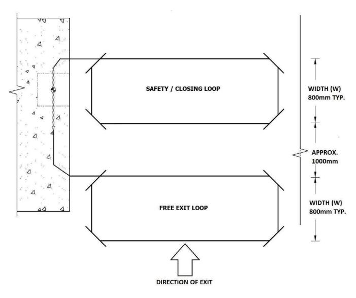
Figure 50: Loop installation for free exit
