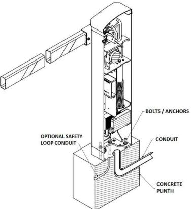
Figure 21: Isometric Section
