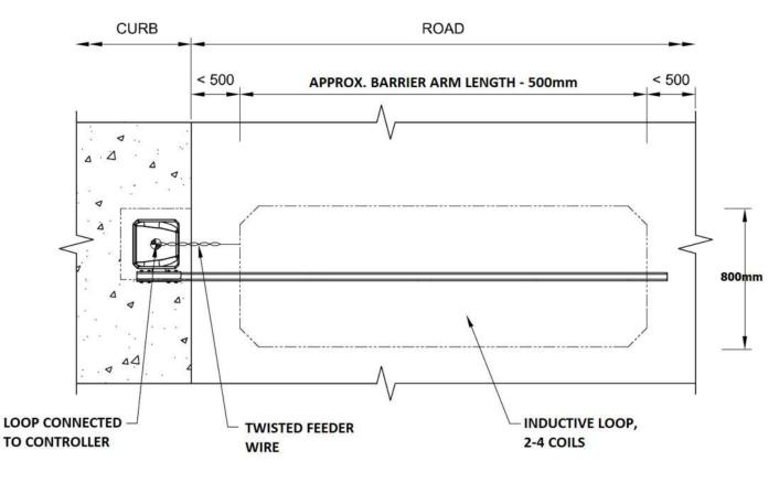
Figure 24: Typical Safety/Closing Loop
