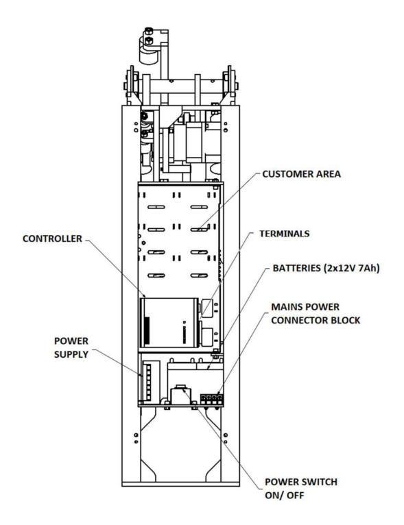
Figure 2: Electronic Components
