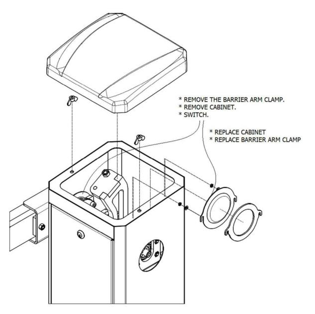
Figure 44: Removing the End Cap
