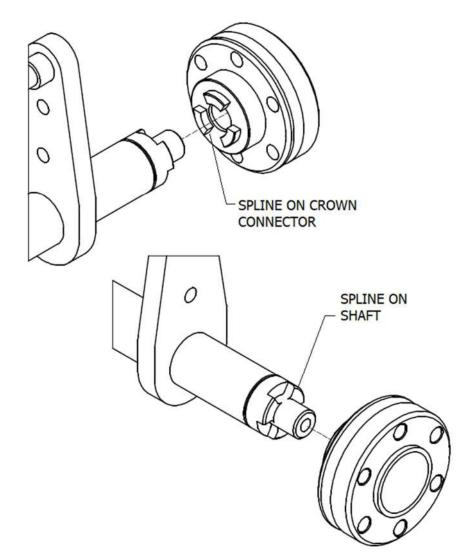
Figure 34: Spline between crown connector and shaft
