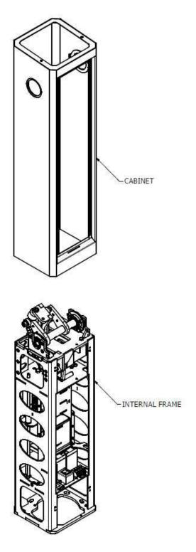
Figure 28: Removing the Cabinet
