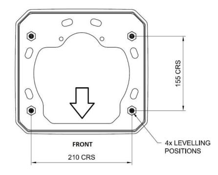
Figure 31: Frame Levelling Adjustment
