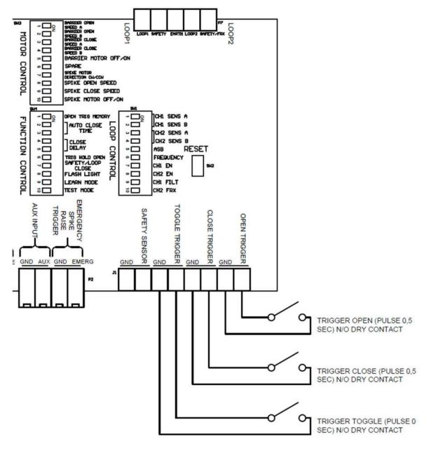
Figure 9: Triggers & Inputs
