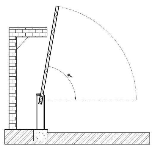
Figure 38: Opening limitation required on barrier arm
