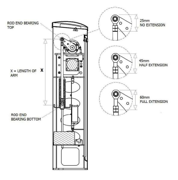
Figure 16: Adjusting Spring Tension
