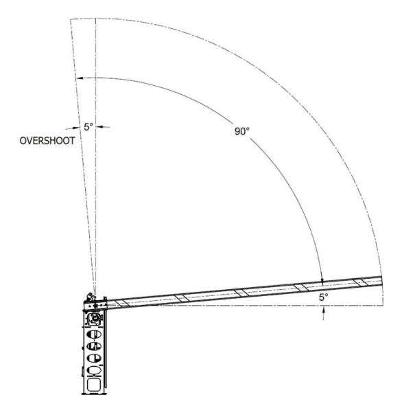
Figure 37: Arm shown in 90-degree operation and apparent overshoot
