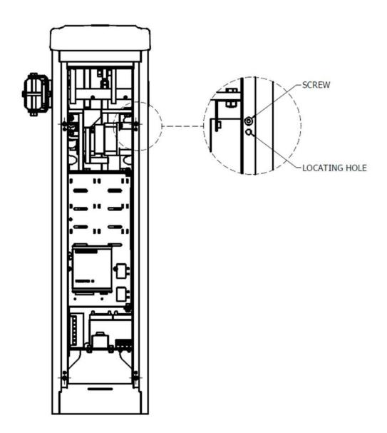
Figure 29: Locating holes and bolting positions
