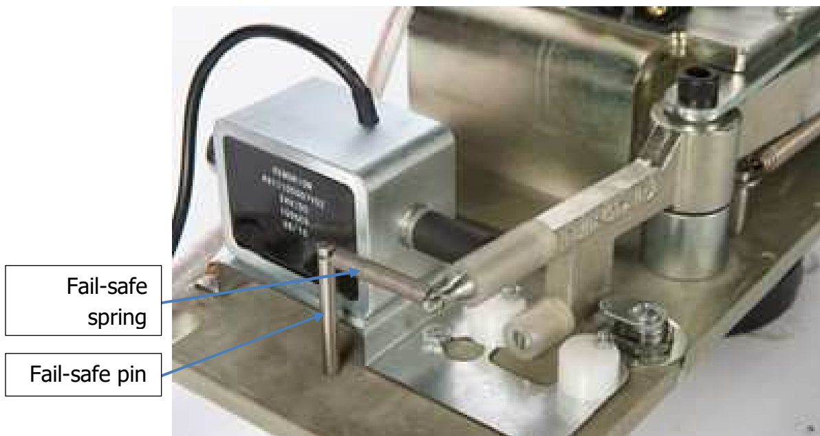
Figure 28: Solenoid in Fail-safe arrangement
